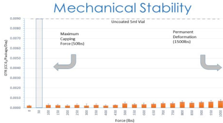
Barrier coating performance maintained well above normal capping force.
